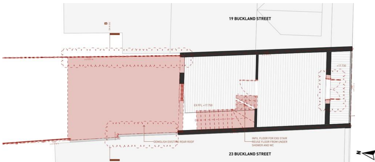
Figure 9: Proposed first floor demolition plan
