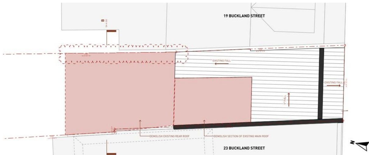
Figure 10: Proposed second floor demolition plan
